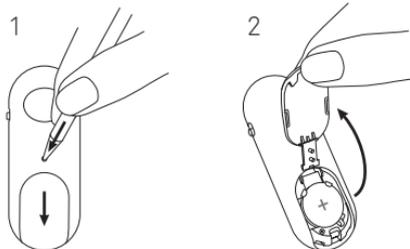
Remove the battery from the battery compartment
