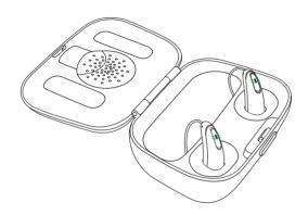
The charging process will automatically stop when the batteries are fully charged, so the hearing aids can be safely left in the charger. It can take up to 3 hours to charge the hearing aids. The charger cover can be closed while charging.
