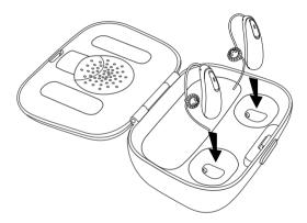
• Make sure the left and right hearing aid markings match the left (blue), right (red) indicators next to the charging slots. 2. The indicator light on the hearing aids will show the charging state of the battery until the hearing aids are fully charged. When fully charged the indicator light will remain on, i.e. solid green light.
