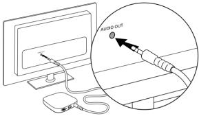
① If your TV loudspeakers switch off when connected with the analog 3.5mm audio cable, use the optical audio cable instead (see Optional: Connecting with optical cable).
