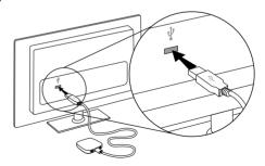
When the TV Connector is plugged into a power source for the first time, the connection to the hearing aids will be automatic. The hearing aids will play a confirmation melody when the connection is successful.
