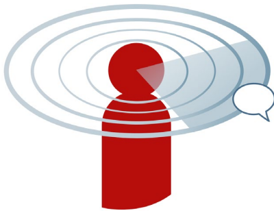
Figure 1. When speech is detected from the front , Dynamic SpeechBeam focuses the directional beam to the front.
